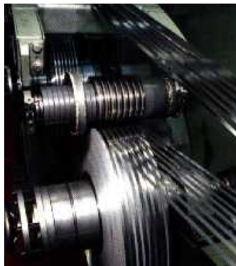
Cold rolled coil being split into narrow strips
