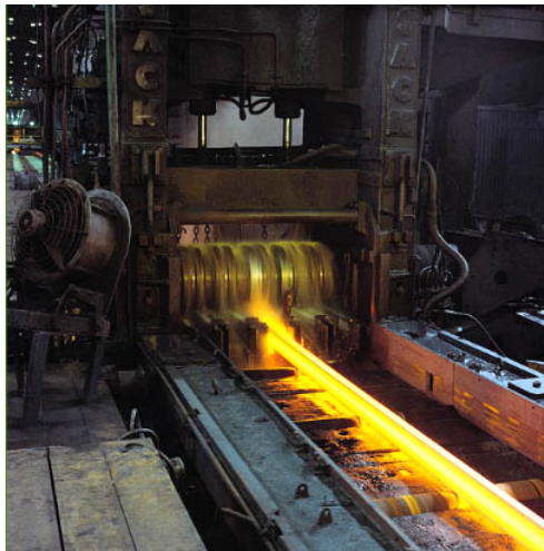
Rolling of Rails
