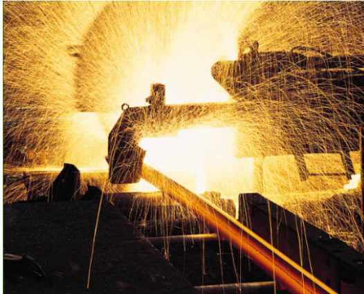
Hot Cutting the rolled Rails
