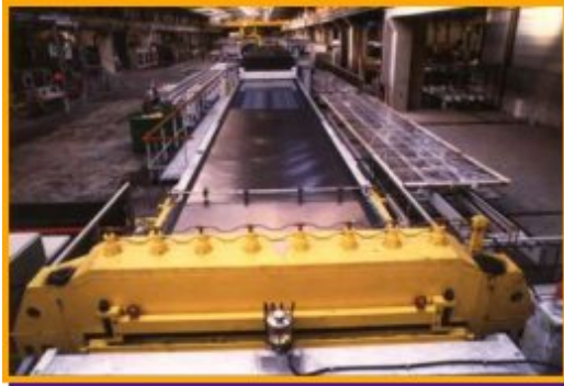
Al Sheet being rolled out
