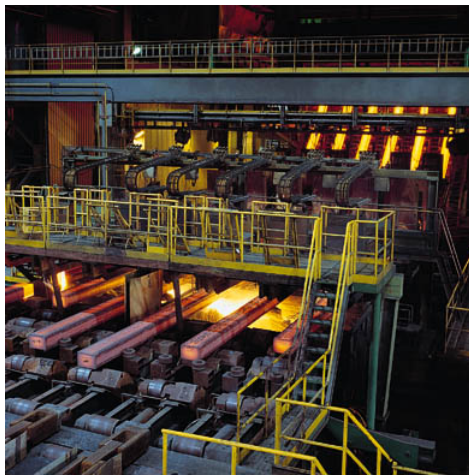
Continuous Steel Casting Line rolling out billets
