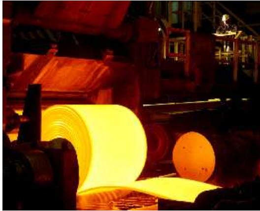
Hot rolled strips being coiled
