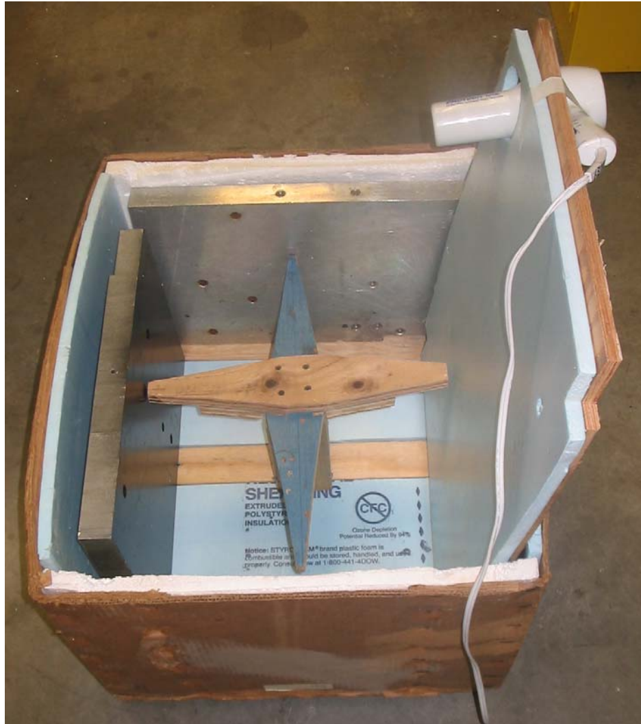
Figure 2. Photo of Experimental Apparatus for Heating the Aluminum Plates
