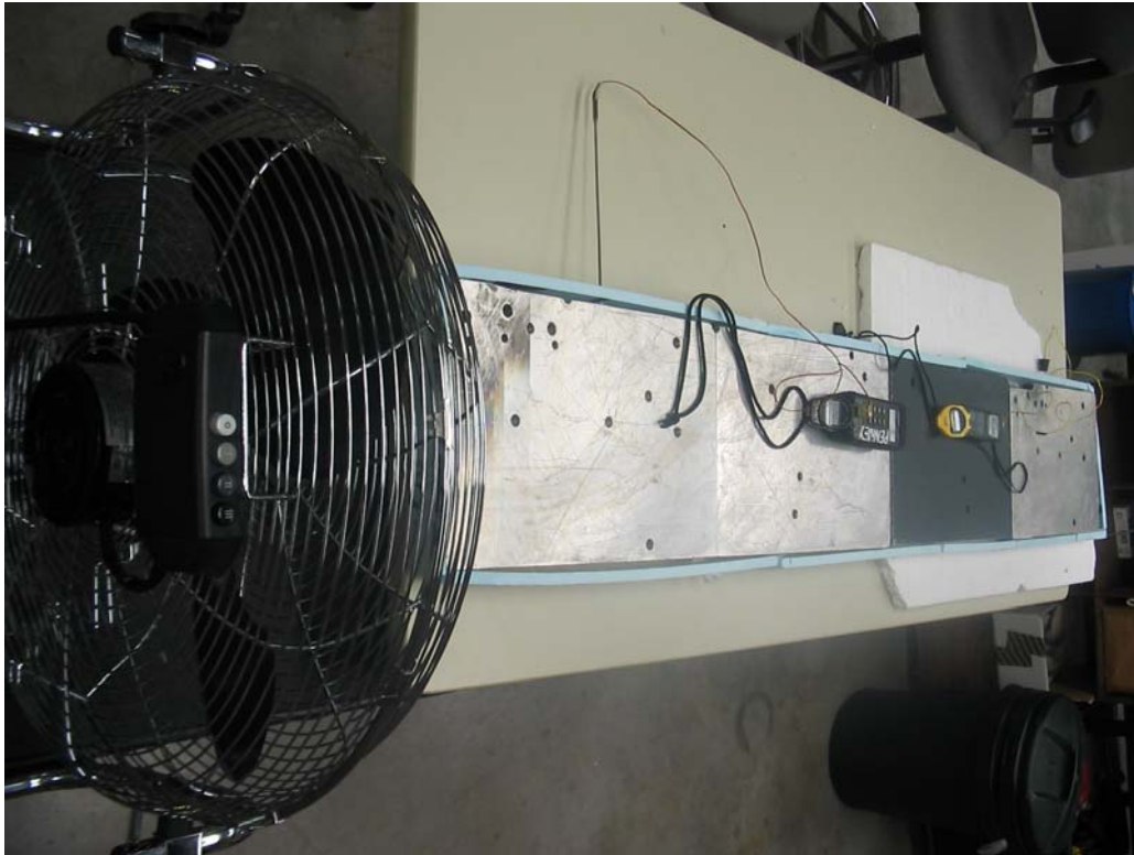
Figure 4. Experimental Apparatus for Determining the Heat Transfer Coefficients.
