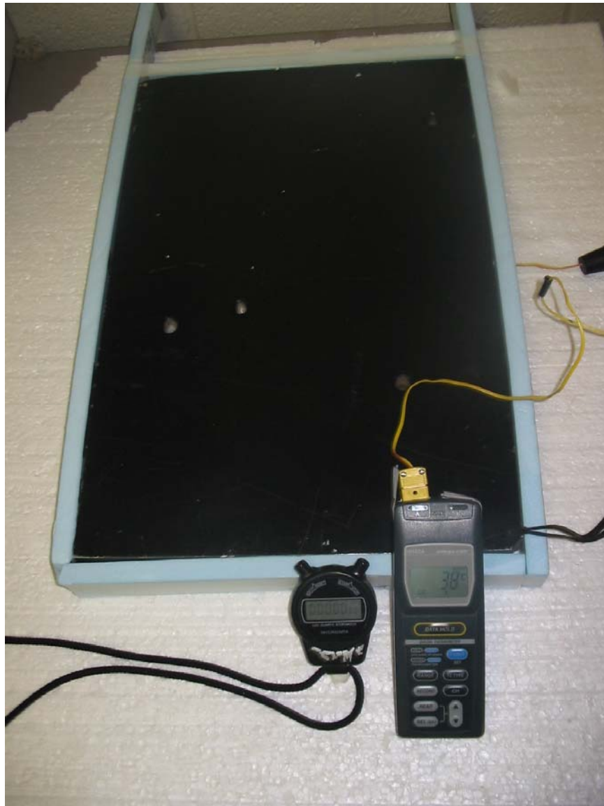
FIGURE 4. Aluminum plate cooling apparatus. Stopwatch and Thermocouple/reader are shown.
