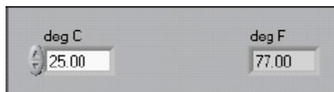
LabVIEW creates corresponding control and indicator terminals on the block diagram. The terminals represent the data type of the control or indicator. For example, a DBL terminal, shown at left, represents a double-precision, floating-point numeric control or indicator.
