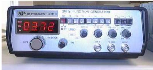
Figure 3. BK Precision 3011B Function Generator
