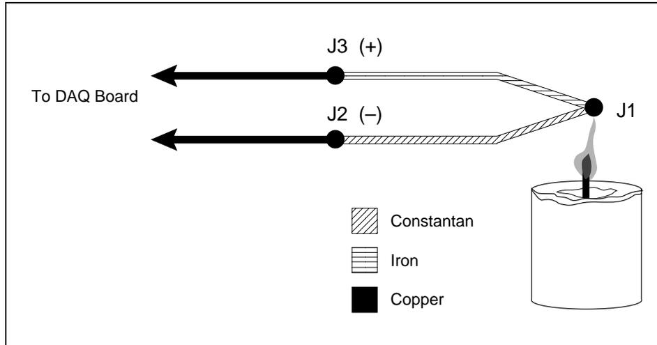
Figure 2. J-Type Thermocouple
